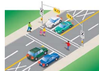
Marked pedestrian crosswalks
